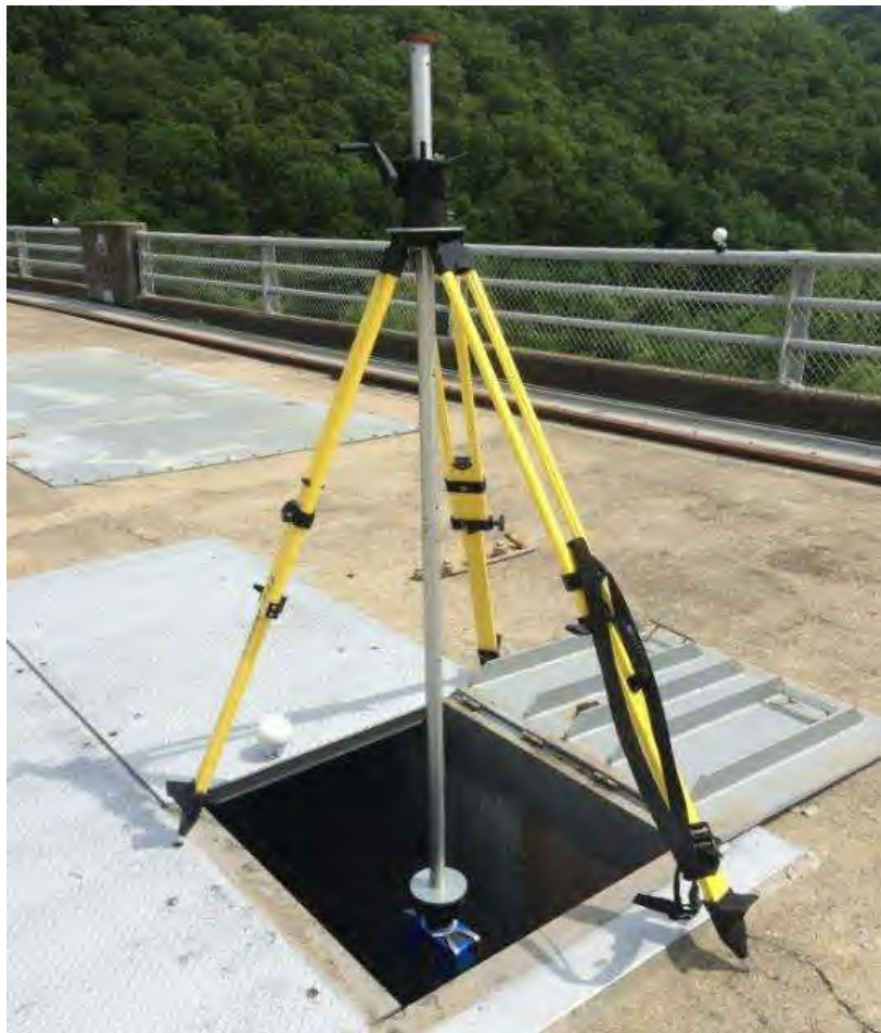
Figure 10-2. A Faro scanner set up inverted for data collection. (USACE Huntington District).
