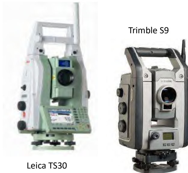
Figure 3-1. Leica TS30 and Trimble S9 are example of electronic total stations that can be used for high precision machine alignment and deformation measurements. Accuracy specified at 1.0 mm (distance) and 0.5 sec (angular).
