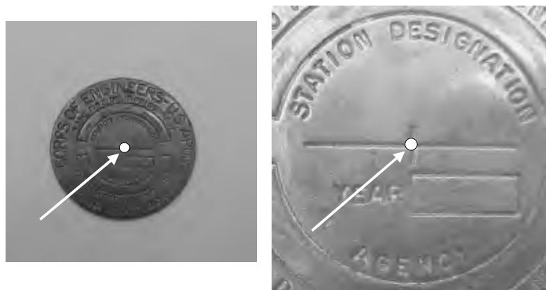
Figure 4-3. Comparison of optical plummet centering devices. The left-hand image shows the field-of-view and centering circle for a standard optical plummet fixed-mounted in a tribrach. The right-hand image shows the greater magnification and centering ability provided by a nadir plummet instrument. Both images show the same brass disk at an instrument height of approximately 1.5 m.
