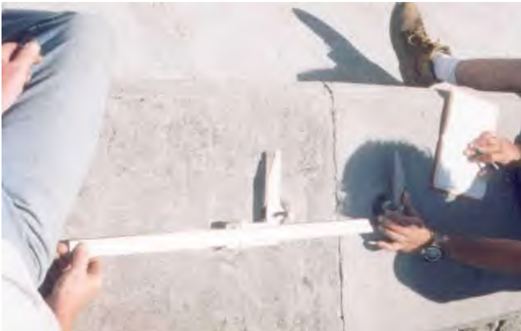
Figure 7-5. Starrett vernier caliper crack measurements between monoliths. Central & Southern Florida Flood Control Project (Jacksonville District and Arc Surveying & Mapping, Inc).
