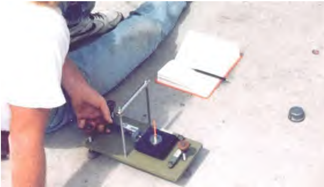
Figure 7-1. Alignment micrometer measurements relative to fixed baseline.
