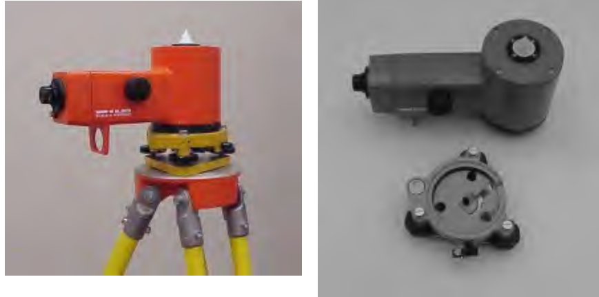
Figure 4-2. Nadir plummet instrument from Leica Co. Nadir plummets operate like an automatic level but establish a vertical LOS. The tribrach is centered over the surveyor's mark using the nadir plummet. Then a theodolite or a GPS antenna is placed in the tribrach by forced centering.
